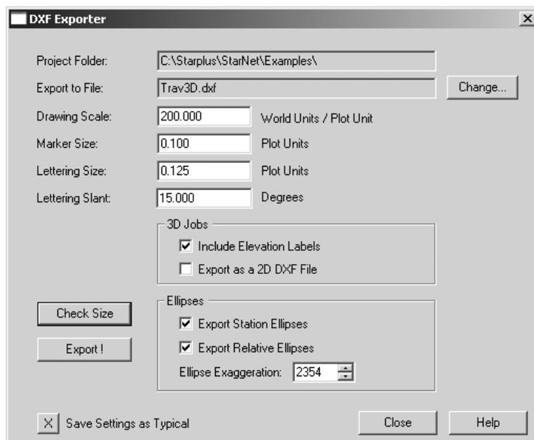
The DXF Exporter will produce a DXF file that can be used to transfer a scaled plot of a project into AutoCAD or compatible graphics software packages. By default, the file is given the name of the project, however you can change it to whatever you want.
