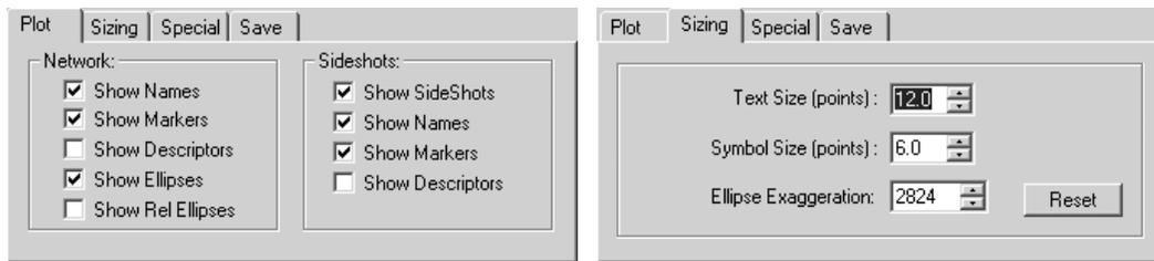
The “Special” tab shown below includes options useful when viewing certain types of plots. For example, the “Show Only Fixed Names and Station Markers” option shows only your “fixed” control points in a network plot.
